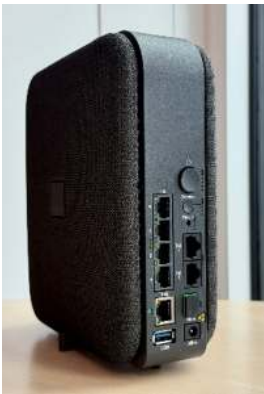
Raised indicators on the back of the Livebox 7 help visually-impaired users to locate buttons and ports by touch.
